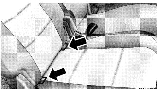
**Second Row Right Side Installing the LATCH-Compatible Child Restraint System**
